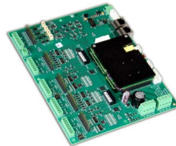
Figure 8 - Dxl/O™ development board with one DZE plug-in servo drive module and multiple I/O points
