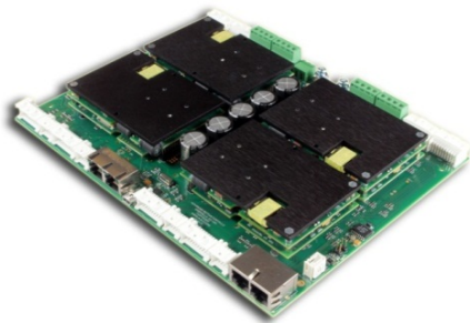
Figure 7 - DxM™ mounting card with one DZE and three DZS servo drive plug-in modules
